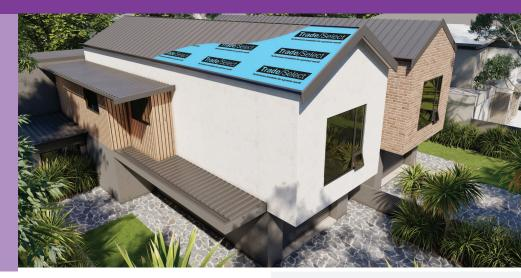
Trade Select<sup>™</sup> Sarking xR is a Extra Heavy Duty double-sided radiant barrier, designed for use under metal deck roofs where temperatures can exceed 80°C, and with battened out cladding to create an extra reflective air space for enhanced R-Value. It is an Air and Water Barrier, Class 2 Vapour Barrier product, suitable for use in all roof and wall applications.
