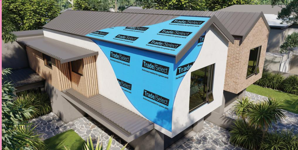
Trade Select™ Sarking xR HD is a Heavy Duty double-sided radiant barrier, designed for use under metal deck roofs where temperatures can exceed 80°C, and with battened out cladding to create an extra reflective air space for enhanced R-value. It is an Air and Water Barrier, Class 2 Vapour Barrier product, suitable for use in all roof and wall applications.
